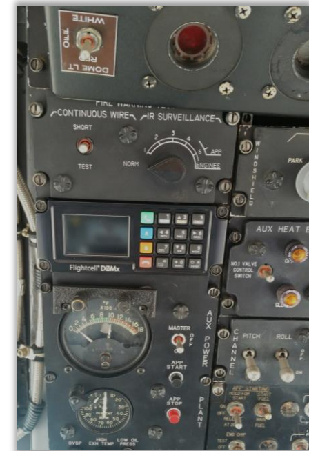
Flightcell DZMx Installed in the Cockpit
